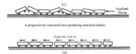
A uniformly applied force shared by the structure. By this simple principle there is no limit to which the structure may be accelerated or decelerated. Fig 19.
