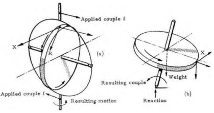
Fig 51. The dynamics of a spinning top.
