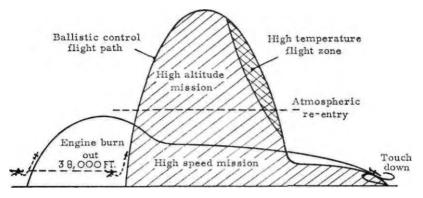
Fig 1. Basic flight programme of the X-15.
