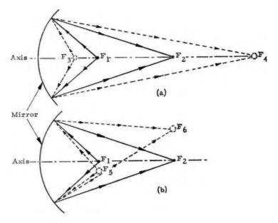
Fig 54. The fundaments of optically focusing a beam of light to a variable focal length.
