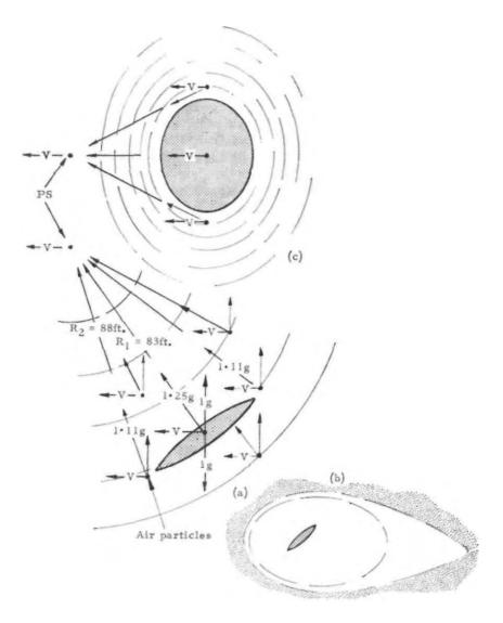
Fig 34. Atmospheric displacement in a moving G. field due to translational velocity and acceleration towards point source.
