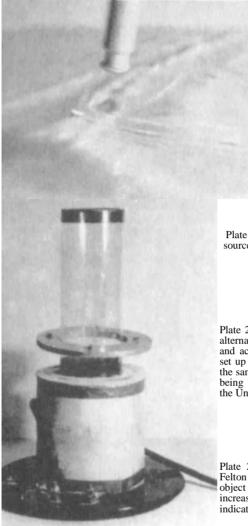
Plate 27. Water analogy of repulsion point source taking surrounding medium along with disc.
