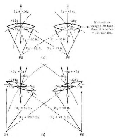
Fig 84. Two R field craft in hovering attitude, each craft producing 20 per cent of the lift force of the other.
