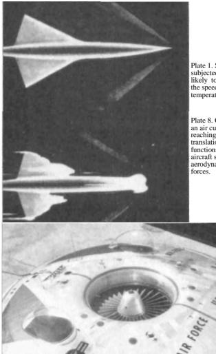
Plate 1. Stainless steel model subjected to air blast conditions likely to be met at five times the speed of sound. The temperature is about 3,000F.
