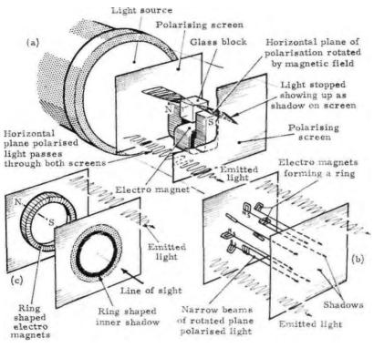
Fig 46. Illumination of a Magnetic Field due to rotation of the plane of polarisation.
