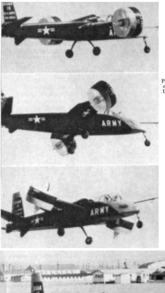
Plate 4. VTOL sequence of the experimental DOAK aircraft with ducted swivel rotors.
